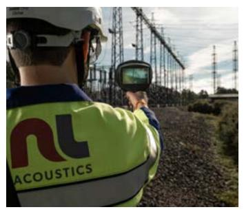
The NL Camera is an easy-to-use, stand-alone device for detecting and localizing partial discharges (PD) in medium- and high-voltage electrical systems during routine inspections. The NL Camera utilizes 124 microphones to detect and locate sounds emitted by partial discharges – even when they are completely inaudible to the human ear. PDs begin emitting sound before components start to heat up, and the NL Camera enables problems to be detected at an early stage.
